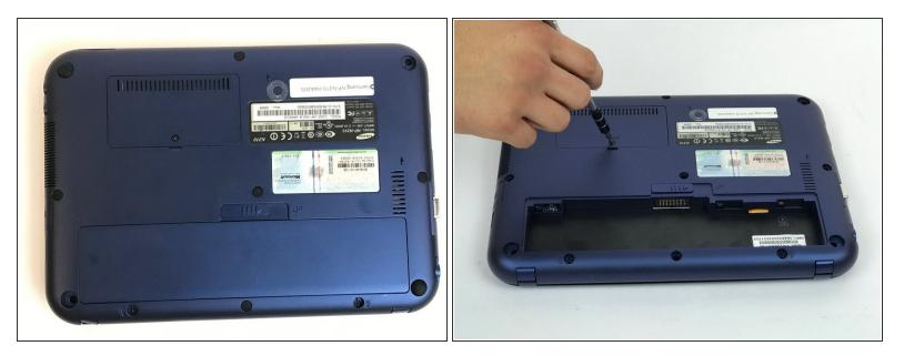
Locate, and unscrew the 11 Phillips 8mm back cover screws, and 1 Phillips 5mm screw on the RAM cover. Use a #1 Philips screw driver to remove the screws.
