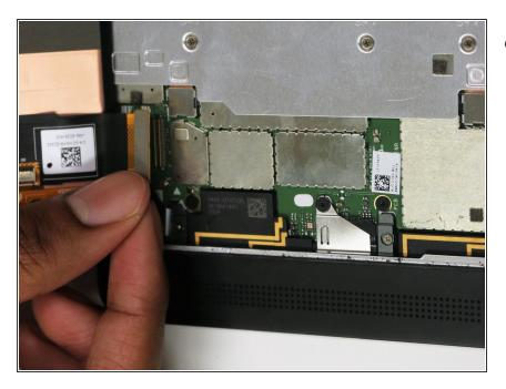
Disconnect the connector from the tablet.
