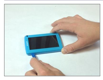
Pry the seam between the screen and the case and slide it on all four sides with a large plastic opening tool until the plastic case comes off.
