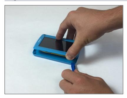
• Lift the device off of the case and flip over the device so that it sits screen side down.
