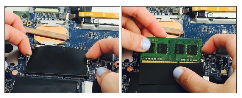
Pull the two metal brackets out away from RAM unit while simultaneously sliding the RAM unit out.
