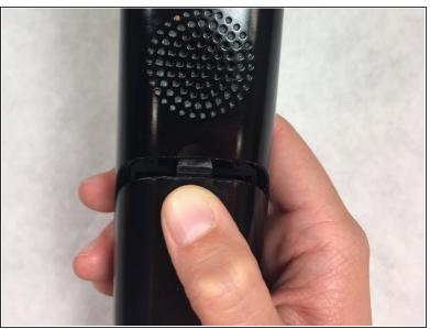
Slide the back cover down towards the bottom of the phone to remove.
