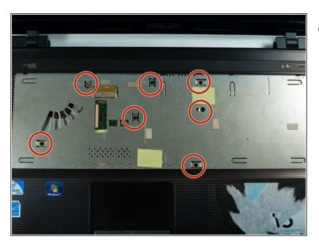
Flip the laptop over and remove the seven 5mm Phillips #1 screws.
