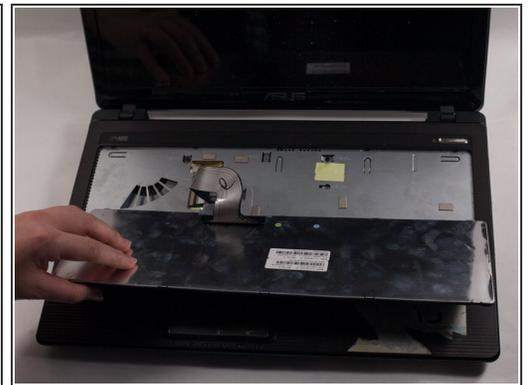
**⚠** There is a ribbon connector underneath the keyboard. When lifting up the keyboard be gentle and carefully it up.
