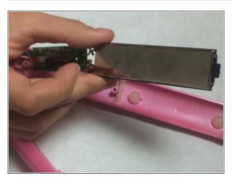
Lift plate and circuit assembly away from flat iron case.
