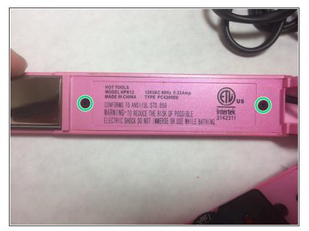
Flip device to access the non-control assembly flat iron arm and remove two 3.5mm "J0" screws that attaches cover to flat iron base.
