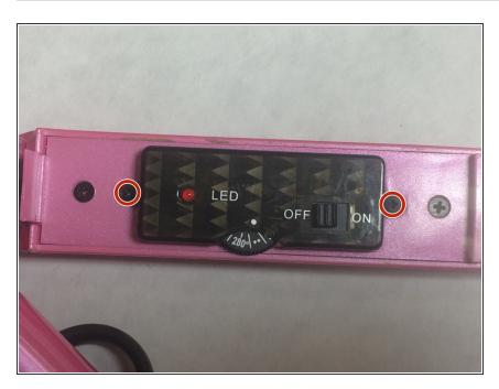
Use the JIS #0 screwdriver to remove the two 3.5mm "J0" screws that attach the control assembly cover to the flat iron base.
