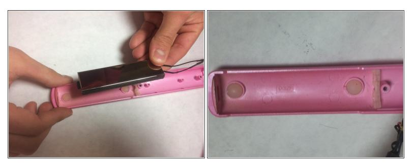
Lift heating plate away from flat iron case.
