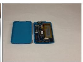
Insert the plastic opening tool into the groove between the two halves of the cover. Pry the two
