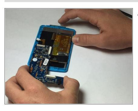
Now remove the motherboard and all of the connected components.
