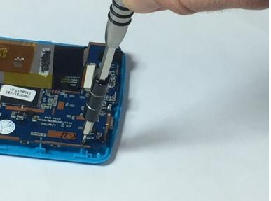
Using the ph#00 screwdriver, remove the four 5mm screws that connect the motherboard to the casing.
