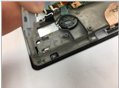
Peel up the tape securing the assembly.
