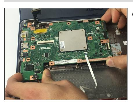
Lift the motherboard up and out of the chassis.
