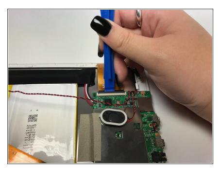
Using the plastic opening tool, lift up the black retaining flap that secures the display ZIF (zero insertion force) ribbon connector to the motherboard.
