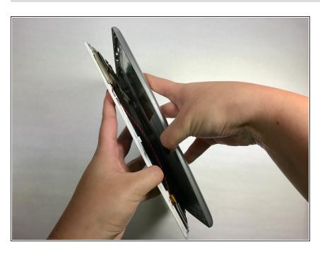
Using an unfolding motion along the top edge of the tablet, carefully separate the front panel from the back case.
