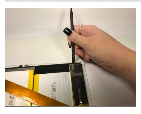
Lift the screen from the front panel with a prying motion to detach it from the clips holding it in place.
