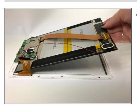
Lift the screen from the front panel to remove.
