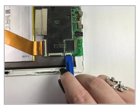
Using the plastic opening tool, lift up the black retaining flap that secures the volume and power button ZIF (zero insertion force) ribbon connector to the motherboard.
