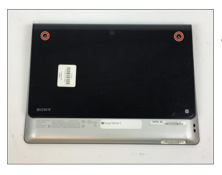
Remove the two 10mm Phillips #0 screws located under the grips.
