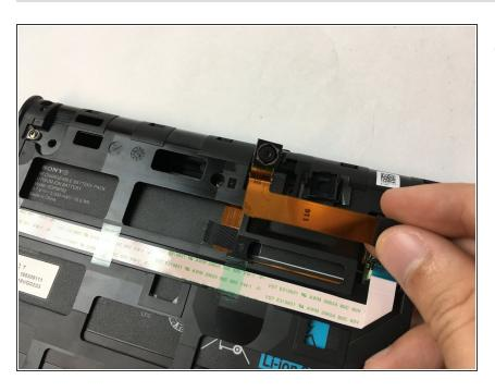
Remove the assembly from the plastic shielding.
