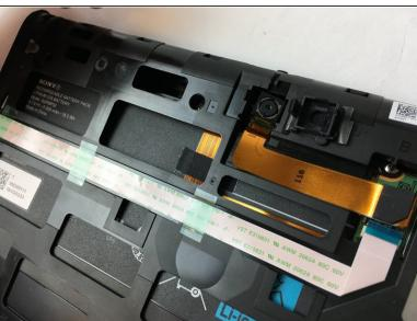
Use a finger or a spudger to pull on camera housing.
