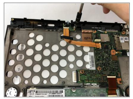
Remove the single 5mm #0 Philips screw.
