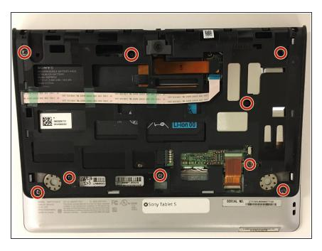
Once the casing is off, remove the nine 5mm Phillips #0 screws shown.
