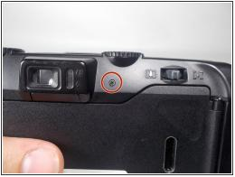
Remove the 5 Phillips screws from the sides and the back.
