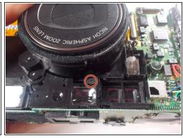
Use a JIS #0 screwdriver to remove the three marked screws found around the perimeter of the lens.
