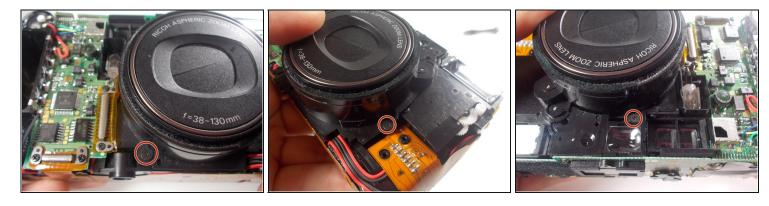
• Use a JIS #0 screwdriver to remove the three marked screws found around the perimeter of the lens.
