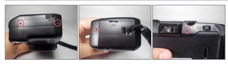
• Remove the 5 Phillips screws from the sides and the back.
