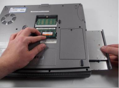
While holding down the switch in the RAM compartment, pull out the CD Drive.
