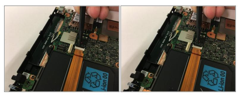
Use a spudger to lift the zero insertion force connector latch for the long ribbon cable to the right of the battery, then pull the cable loose from its socket.
