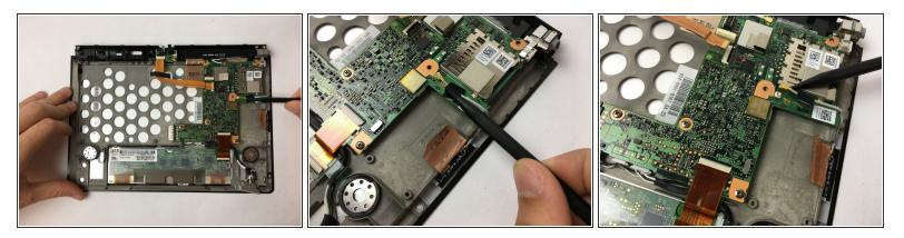
• Use a spudger to carefully remove the black tape, and gently disconnect the pin connector.
