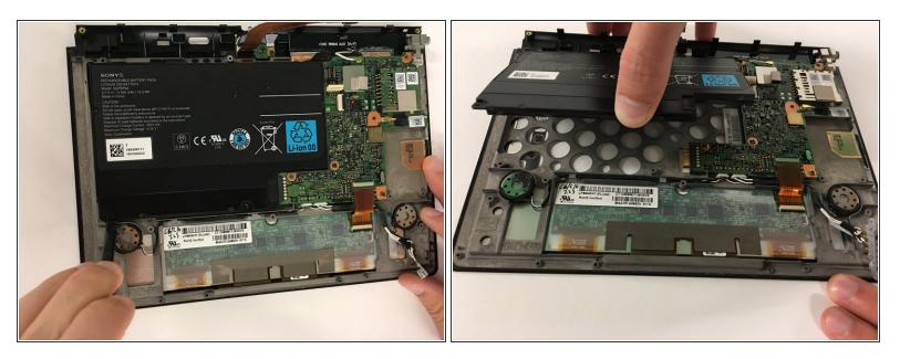
• Use the spudger to pop the battery loose and remove the battery.
