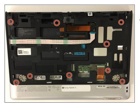
Once the casing is off, remove the nine 5mm Phillips #0 screws shown.
