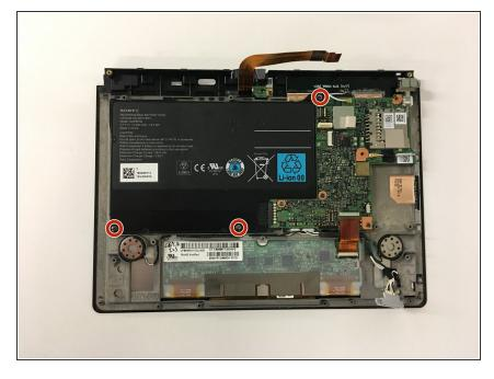
Remove the three 5mm Phillips #0 screws securing the original battery.
