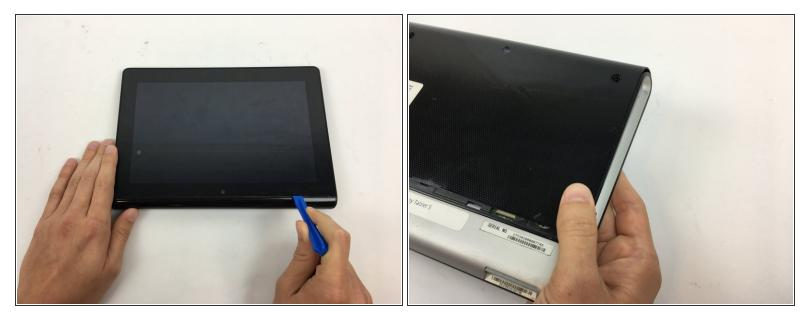
Flip the tablet over and use a plastic opening tool to pry the casing away from the top of the screen. Push the back cover off.
