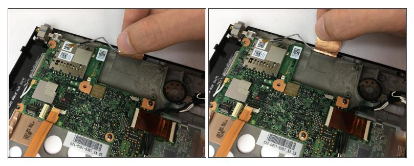
• Remove the copper tape securing the Wi-Fi antenna.
