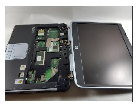
Completely remove the keyboard from the rest of the laptop. To reassemble your device, follow these instructions in reverse order.
