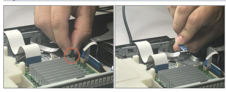
Now, pull the small ribbon cable that connects between the motherboard and the Bluetooth module.
