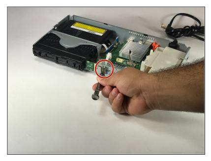
Use your Phillips screwdriver to remove the silver screw holding the Bluetooth module in place.
