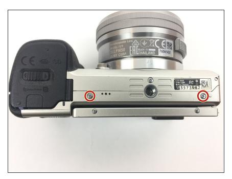
• Turn the camera upside down and unscrew these two bottom 6 mm screws located on either side of the body by using the J00 head screw.
