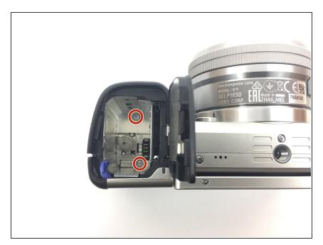
Locate the two 4 mm screws within the battery compartment and unscrew them using the J00 screw head.
