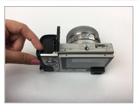
• Push the latch back to release battery.
