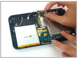
• Using the spudger, disconnect the front camera by lifting up on the connector.
