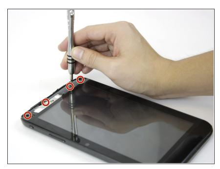
Using the Torx screwdriver, remove the 4mm screws.
