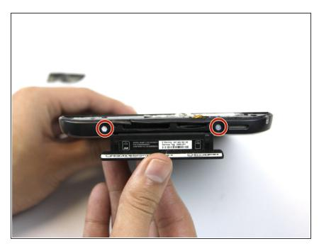
With the Torx screwdriver, remove the two 5mm screws.
