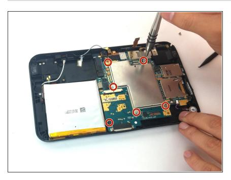
Using the Torx screwdriver, remove the six 3mm screws.
