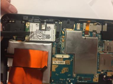
With the spudger, disconnect the antenna cable located on the module.
