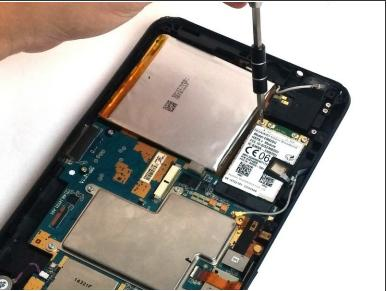
Remove the two 3mm screws securing the GSM module. Use the Torx screwdriver.
