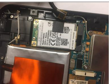
Using tweezers, remove the tape connected to the GSM module.
