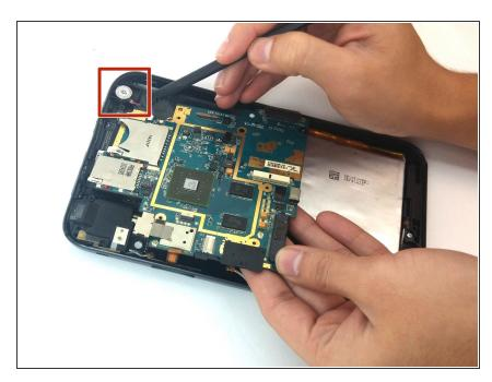
Use the spudger to lift the vibration motor out of the case.
