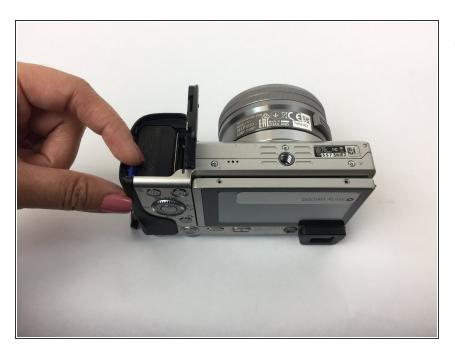
Push the latch back to release battery.
