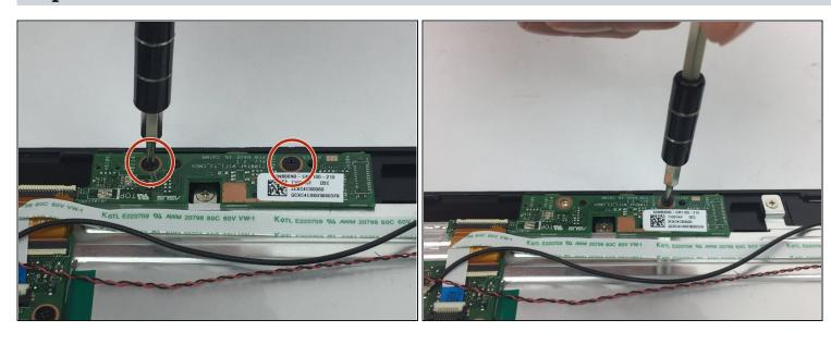
• Remove the two 4.0 mm black screws from the camera board.
