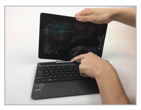
Detach the keyboard from the screen by depressing the silver button on the tablet's hinge and pulling upwards on the tablet.
