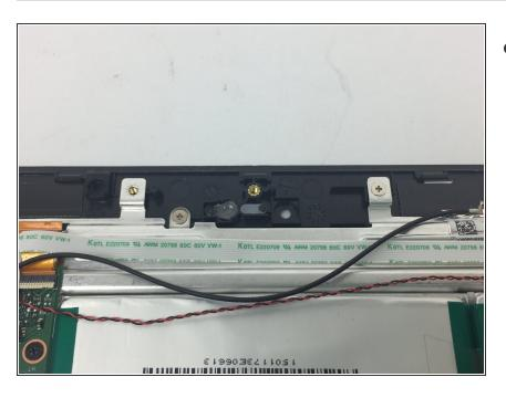
Lift the camera board away from the device.
