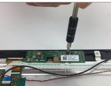
Remove the two 4.0 mm black screws from the camera board.
