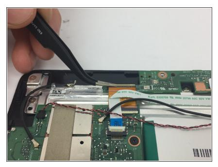
Using tweezers, disconnect the orange ribbon cable from the camera board by lightly pulling it up and towards the motherboard.
