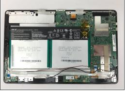
Insert the spudger behind the plastic backing of the tablet and then slide the spudger around the outside of the tablet, carefully releasing all internal clips.
