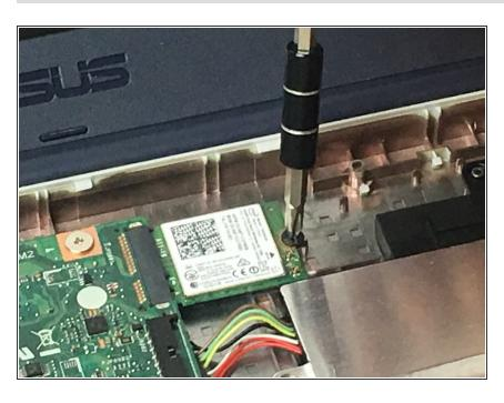
Unscrew the single 4 mm Phillips #1 screw pinning the wireless card in place.
