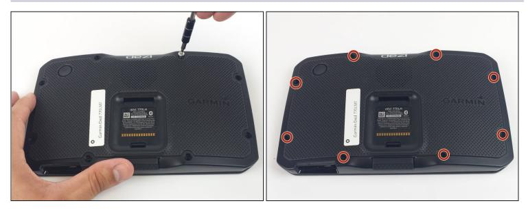
• Turn the device screen down and using the screwdriver remove all eight screws from the back plate.
