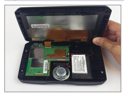
• Use the spudger to pry apart the screen from all around the device.
