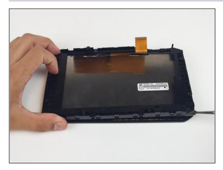
Once the screws have been taken out, use a spudger to carefully remove the cover.
