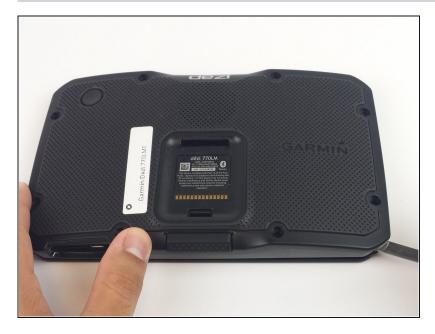
Place a nylon spudger in the seam between the front and back panel and carefully lift around the edge of the device.
