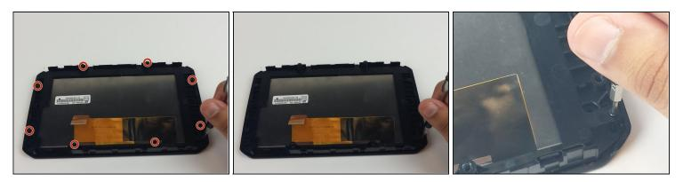
• Now you have the screen, which is enclosed by another cover. Remove the eight screws that hold it in place.
