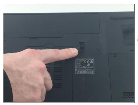
This latch holds your battery in place, it should always be locked.
