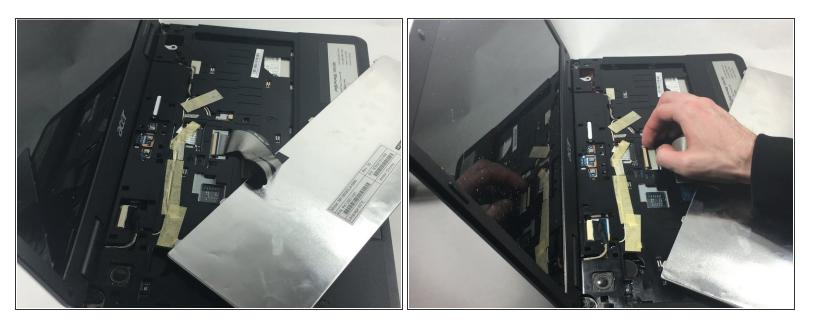
• Disconnect the keyboard flex cable, and now you are ready to install a new keyboard.
