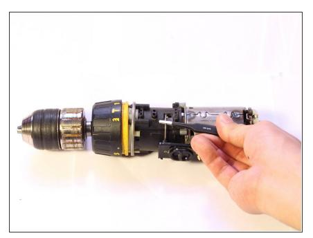
• Using the tweezers, grab the metal leg on either side of the switch and lift it outwards from the case.
