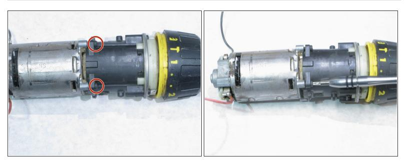
Use a Torx T10 screw bit to remove the four 11mm screws around the motor.
