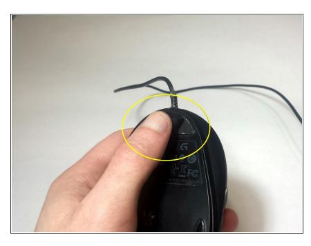
Remove the top mouse foot using a Jimmy and the same technique as in Step 1.
