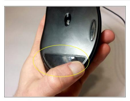
Use a Jimmy to remove the mouse feet. Be careful to remove any film left by the mouse feet as well.
