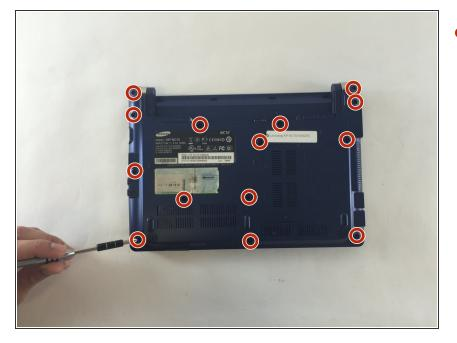
Remove all 14 of the 3.93 mm screws using a PH1 screw bit.
