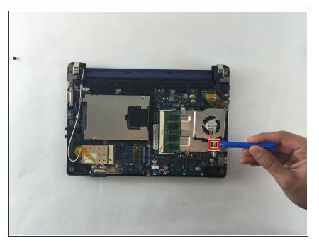
Unplug the wires connected to the fan using a plastic opening tool.
