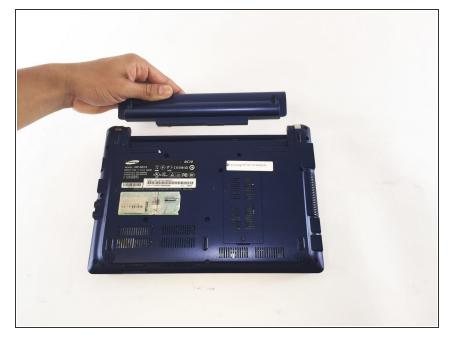
• Pull the battery up from the device.
