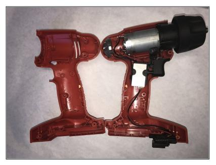
Separate the outer drill case to expose the components and switch.
