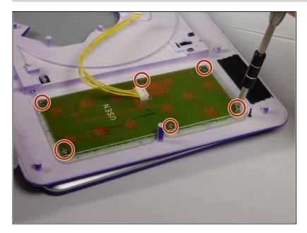
Use a Philips Head screwdriver to remove six 5mm screws.
