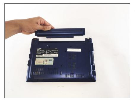
• Pull the battery up from the device.
