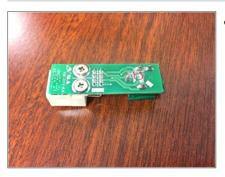
The center pin is located where the red circle is at on the picture
