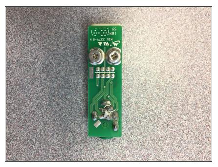
Soldering does not have to be perfect as long as it connects the two pin we located in the previous picture.
