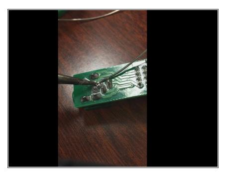
Hold the soldering gun in one hand and the solder in another. Lightly touch them together where the pin is shown in previous step.
