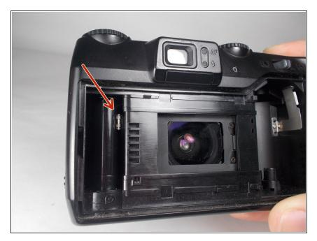
Then, insert the unrolled part of the film into the slot on the left part of the compartment making sure the silver lever is securing the film.
