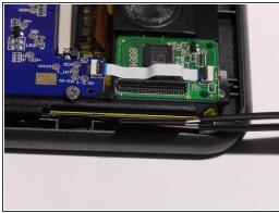
• Lift the black tab and then remove the wire belt.
