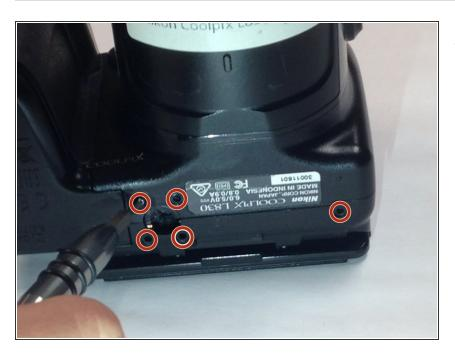
Unscrew the five 3.0mm Phillips #000 screws that are located on the bottom side of the camera.
