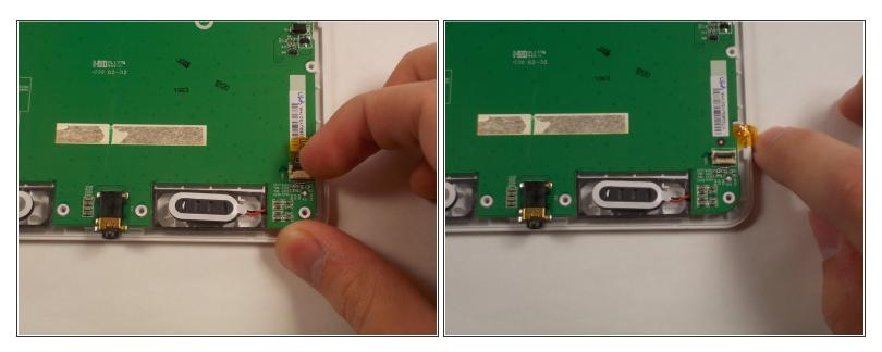
• Use the tip of your plastic spudger or your fingernail to flip up the shorter retaining flap. The smaller gold ribbon cable can now be pulled out safely.
