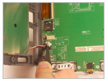
Now, lift up the gray piece, unplug the battery connector, so the gray piece will come free from the rest of the device.
