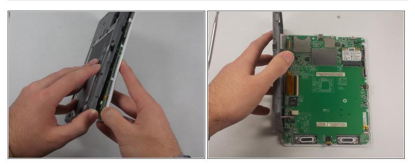
• Carefully pry the back of the device from the front panel and motherboard. There are a series of clips holding them together that need to be separated.
