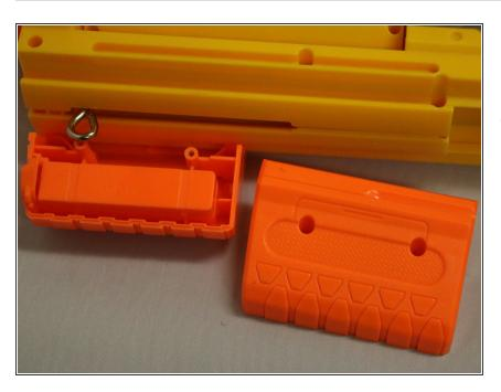
Once screws are removed from the pump part you can then remove the pump parts.
