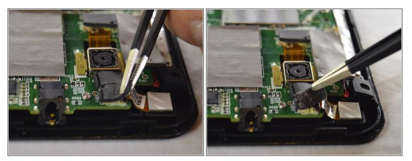
Use the tweezers to remove the black foam stickers from the rear facing camera to expose the wiring.
