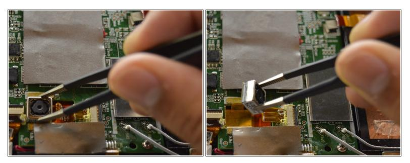
• Using tweezers, lift the camera out from system board.
