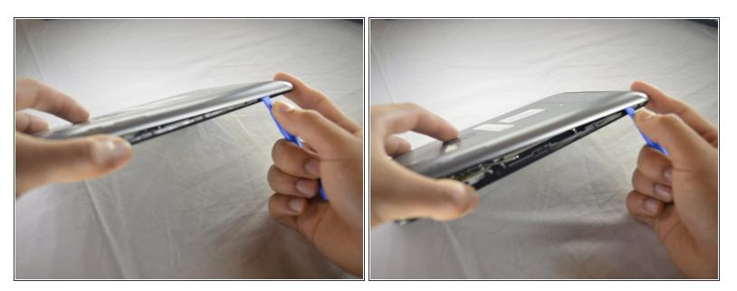
Slide the tool around the perimeter of the tablet until the edge of the cover is completely separated from the display panel assembly.
