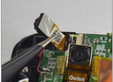
• Lift the camera out from system board and firmly pull the wire out from the connector.
