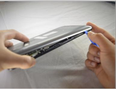
Slide the tool around the perimeter of the tablet until the edge of the cover is completely separated from the display panel assembly.
