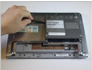
Using a spudger pry the panel up.
