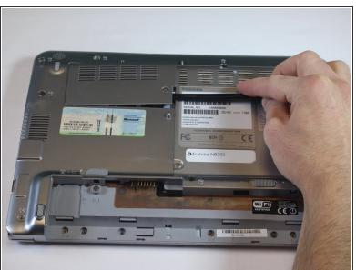
Using a spudger pry up on the open slit next to the screw.
