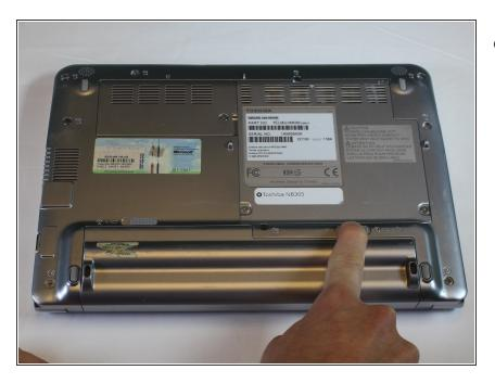
Use your right hand to move latch 1 to the right to unlock the battery.
