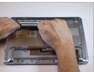
Pull the RAM straight out of the slot.
