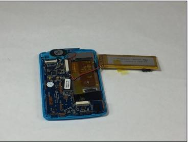
• Wedge a <u>plastic card</u> beneath the battery unit and wiggle the card side to side and up and down gently until the glue sealing the battery to the device is broken.
