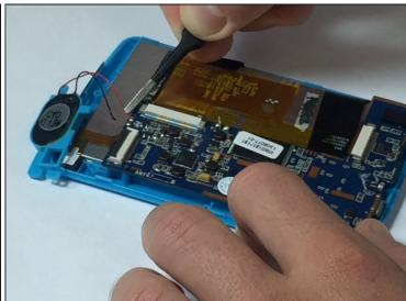
• Solder off the wires connecting the speaker to the device
