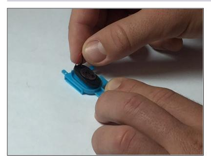
Pull the speaker out of the casing to release it.
