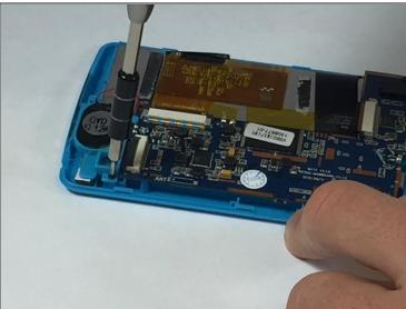
Remove the two 5mm screws attached to the top right and bottom left corners of the speaker
