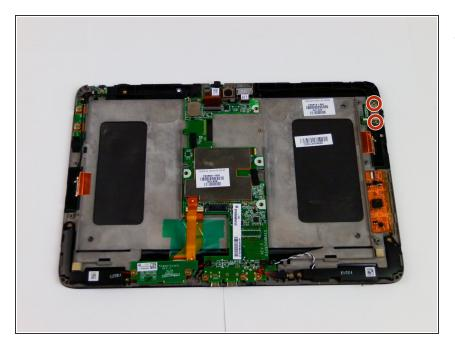
Unscrew the two 3.3 mm screws with a 00 Phillips head screwdriver.
