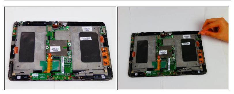
• Remove the metal plate from the audio board.
