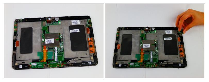
• Remove the audio board from the device.
