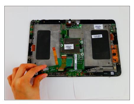
Lift and remove micro card reader board.
