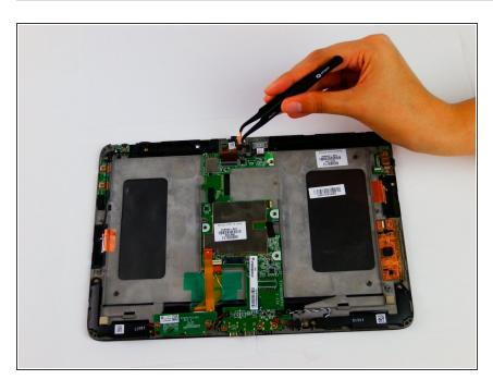
With a pair of tweezers, grab the camera and pull it out of the socket it is in.
