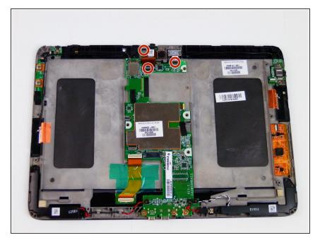
Pull the black plastic security tabs into an upward position.
